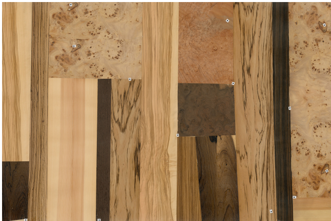
Fig. 9. Scan of the wooden veneer panel used for the results in Section 4. The panel has physical dimensions of 1500 mm × 1000 mm and contains veneer samples from various wood types. The fiducial markers facilitate optical calibration on suitably equipped cutting systems.
