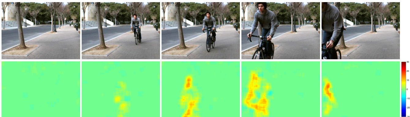
Figure 8: Complex scene with ambient illumination and a large depth range. The velocity is robustly estimated within the range of the illumination (approx. 5m inside), even in outdoor settings.
