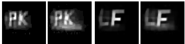
Figure 7. Effects of frame averaging on albedo (left) and geometry (right). The left image in each pair is based on averaging 500 ToF images for each measurement, while the right image in each pair uses only 10.
